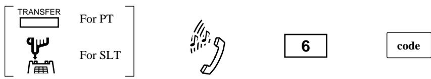
For PT: Press **TRANSFER**. For SLT: Flash the switchhook. Dial tone. Dial **6**. Enter the desired service code.
